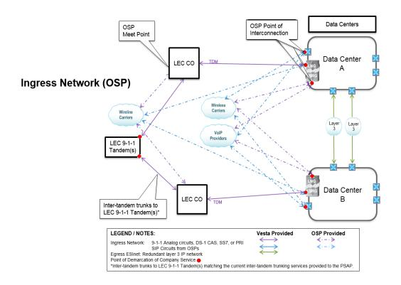
3.1.1.1 Legacy Selective Router Gateways (LSRG's) will provide trunking back to the existing E9-1-1 LEC tandem during the transitional phase. These trunks will allow Call Transfers between the LEC E9-1-1 tandem and the Company's Call routers and vice-versa.
