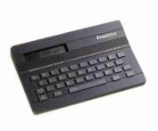
A Motorola application specific IC controls liquid crystal display, logic and a memory of 80,000 words in this hand-held electronic speller from Franklin Computer Corp.
