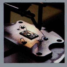
Software engineer uses universal calibration console, which displays engine performance parameters under on-road conditions, to calibrate and test electronic engine control modules.
