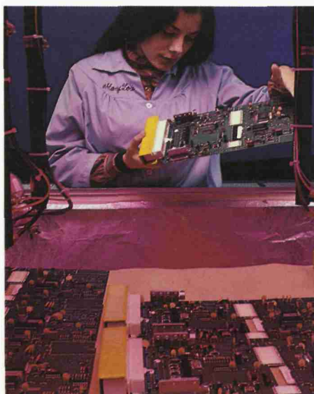
Quality control technician inspects EEC-IV engine control module to ensure proper application of moisture-resistant sealant.
