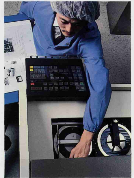
Technician prepares highly automated diamond saw to dice wafers into MC68000 integrated circuit chips. Computerized positioning of the wafer increases production speed and reduces cost.
