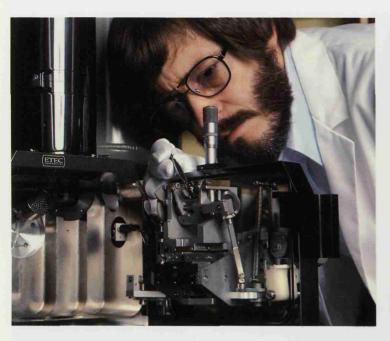
(Above) Electron microscopy makes it possible to pinpoint material flaws, imperfections that earlier would have escaped detection except by stress testing and that could grow into failure mechanisms under severe stress. (Right) A recently installed process performs operating life for zener diodes. With this equipment, one operator can perform operating life and test about one million zener diodes a year.
