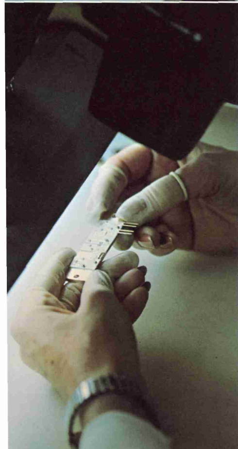
(left) RF Modules are so small and delicate workers must use microscopes during assembly and inspection process.
