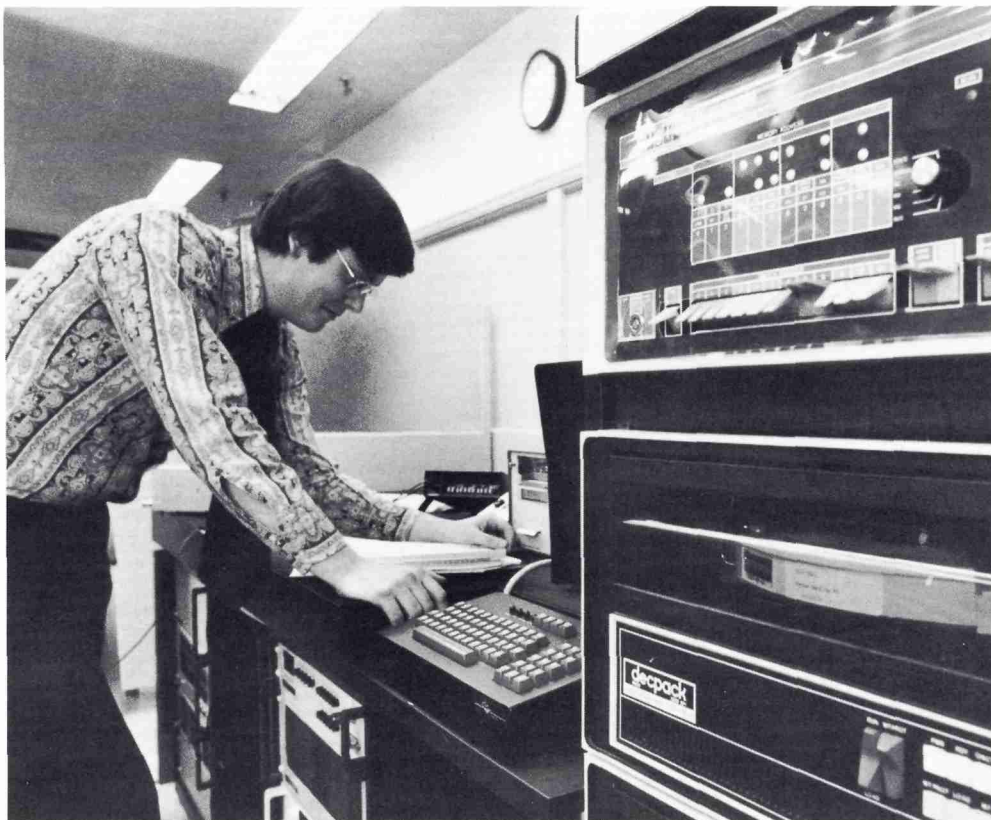
All new Motorola car radios, as well as ignition, voltage regulator and automotive instrument subassemblies, will soon be tested and analyzed by inserting the subassembly into a computer-controlled test system. Here, a Motorola engineer perfects a program for the testing.
