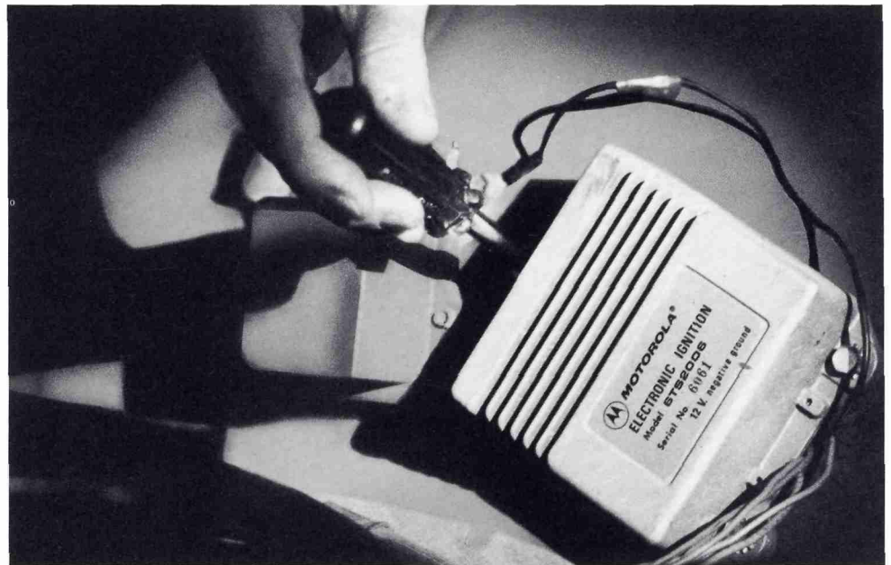
The Motorola-branded aftermarket electronic ignition system is designed for retrofitting in passenger cars, as well as industrial vehicles and engines.
