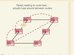
There is always a redundant path inside the network - for the price of one link more than the absolute minimum
