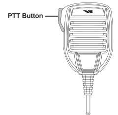
• While a call is in progress, the **PTT** button allows the radio to transmit to other radios in the call.
