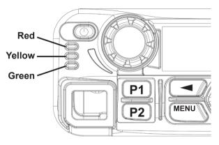
**Blinking red** – Radio is receiving an emergency transmission or has failed the self-test upon powering up.
