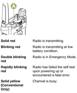
**Blinking yellow** Radio is receiving a secured transmission.
