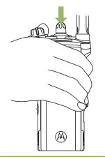
**3** To remove the radio from the carry holder, place the tip of your fingers on the ledge of the carry holder.
