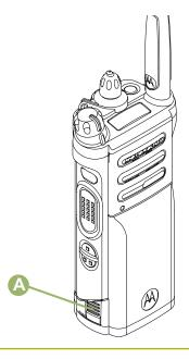
2 To remove the battery, squeeze the release latches (A) at the bottom of the battery until the battery releases from the radio and remove the battery from the radio.
