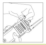
3 Dip the radio completely into the detergent solution and repeat turning action for both knobs, 3-Position A/B/C and the Secure Switch.
