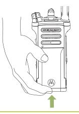
4 Push at the bottom of the radio until the radio is released from it.
