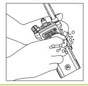
5 Use the toothbrush to lightly brush the gaps at the base of the knobs and around the switches. Take extra care around the Speaker Grill and Microphone port openings.
