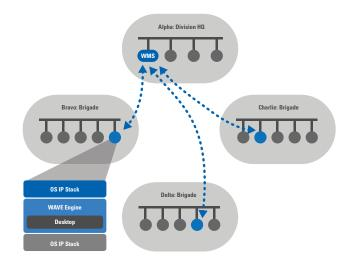
Zones are logical groupings that overlap a network's hardware and connections. Conceptually, Zones exist as a layer between a communications structure (Channels) and a network structure. Zones are discrete and stand alone as a separate layer. They represent the routers and switches and servers in a network, and are configured separately from other communication components of WAVE.
