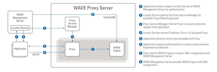
The WAVE Locator Service is an element of the WAVE Management Server and is responsible for assigning an application to an available Proxy Server during sign in and provides it with the address and port of its assigned Proxy Service.
