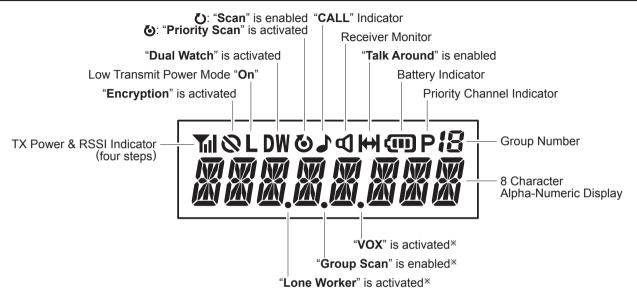
\* These small dot appears continuously until each function is turned "OFF", regardless of the operation of other features.
