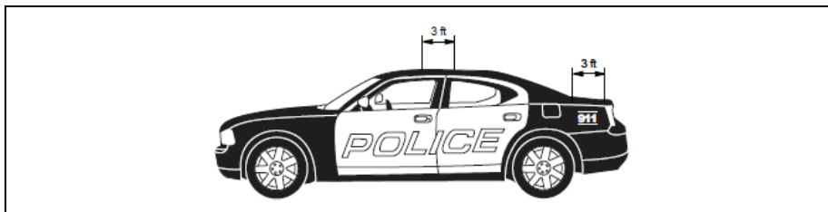
Figure 5: Multiple Antenna Separation
