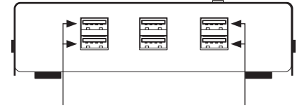
Up to 4 individual VB400 Solo Docks can be connected to the ports shown.
