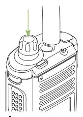
Rotate the **On/Off/Volume Control Knob** clockwise until you hear a click.
