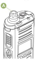
To increase the volume, rotate the On/Off/Volume Control Knob (ⓐ) clockwise.
