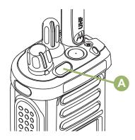
The Top Lightbar indicates the secondary function of MFK and also the status of Intelligent Lighting.
