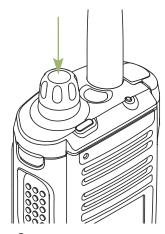
To turn off the radio, rotate the **On/Off/ Volume Control Knob** counterclockwise until you hear a click.
