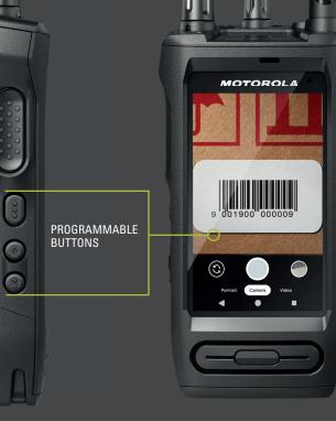
One of the three programmable buttons could be mapped to launch the barcode scanning application.
