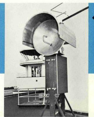
Two-way radio "levels mountains." In the shadow of Mt. Rainer, Aeronautical Radio, Inc. uses Motorola microwave at the Seattle-Tacoma International Airport to beam messages to remote mountain-top aviation radio transmitters.
