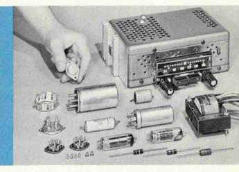
Transistorized power line carrier. Use of transistors in both transmitter and receiver provides greater reliability in Motorola's frequency-shift power line carrier. Even when battery operated during an emergency, this transistorized equipment furnishes dependable, high-speed communication and control facilities for power companies.
