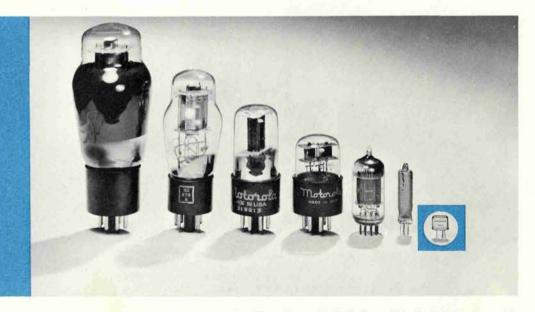
David replaces Goliath. Incredible though it seems, this tiny transistor can perform the functions of a vacuum tube many times its size. Note that through all its evolution, a practical mass-produced vacuum tube has never attained the small size of the transistor.
