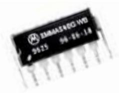
*The MMAS40GWB is Motorola's premier accelerometer sensor for automotive and industrial uses.*
