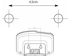
To wall-mount the charger, drill two holes in the wall 3.2cm apart horizontally using an 8mm drill bit.
