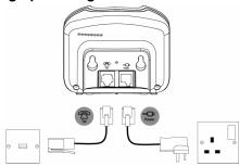
Plug the power adapter with clear connector into the socket marked — on the underside of the base and plug the other end into the mains power wall socket and switch the power on.
