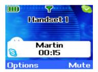
You can turn the microphone back on by selecting Unmute using Soft Key 2 again.
