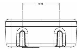
• Insert the wall plugs if necessary, then insert the screws leaving about 5mm protruding from the wall on which to hang the phone.
