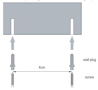
Pull the base/charger out of the stand and slot the holes on the back of the base over the screw heads and gently pull the base/ charger down to make sure it is securely in place.
