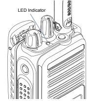
**Blinking red** – Radio is transmitting at low battery condition, receiving an emergency transmission or has failed the self-test upon powering up.
