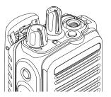
To remove the antenna, turn the antenna counterclockwise. Make sure you turn off the radio and remove the universal connector cover (dust cover) first.
