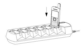
**NOTE:** The battery charging icon will be displayed until the user unplugs the USB cable or takes the radio out of the charger.
