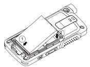
To attach battery cover, align it in place and slide the battery latch until it snaps into place. Slide battery latch into lock position.
