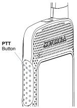
While a call is in progress, the PTT button allows the radio to transmit to other radios in the call.
