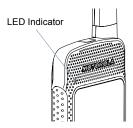
**NOTE:** The LED lights up solid green while the radio is transmitting and double blinks green when the radio is receiving a privacy-enabled call.
