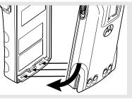
2 Press both sides at the top of the battery against the radio until both latches click into place.
