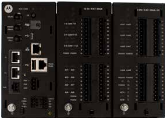
ACE1000 Remote Terminal Unit without cover
