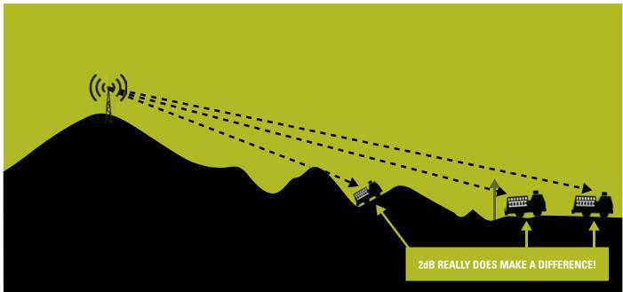
Range in 'typical' systems can be estimated using path loss equations derived by Hata and Okumura propagation model, which was formed as a result of measurements over real terrain in Japan and is used for predicting the behaviour of cellular transmissions. These empirically derived equations are universally
