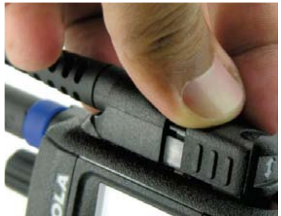
Connector can be detached with one hand in less than two seconds.
