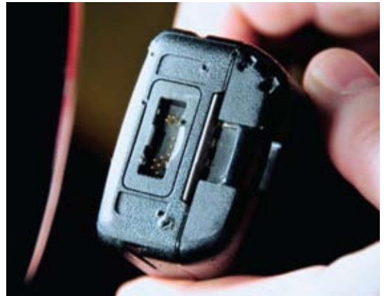
Image shows the bottom of a prototype radio after being dropped onto a bed of nails many times. You can see where the nails have impacted on the radio without bending the pins.
