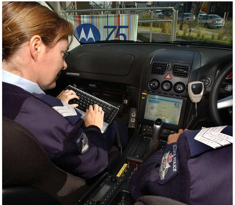
Motorola's solution, a build-own-operate dedicated wireless data communications network, became the centrepiece of a new era in Victoria's emergency services dispatch, response and data capability with police and paramedics able to access the network via in-car touch-screen computers linked to centralised Victoria Police and Metropolitan Ambulance Service databases and dispatch hubs.
