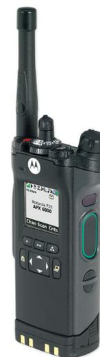
The APX series of trunked radios is available with P25 FDMA and P25 TDMA in the same radio. Dynamic Dual Mode automatically switches between the capabilities.
