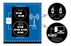
For the software configuration, the TrboX platform which is developed by Shanghai Ji Hua Information System Co., Ltd and based on MOTOTRBO Capacity Plus system now supports the dispatching and controlling function of the terminal intercoms in the airport command centre, and can record all intercom calls within the airport.
