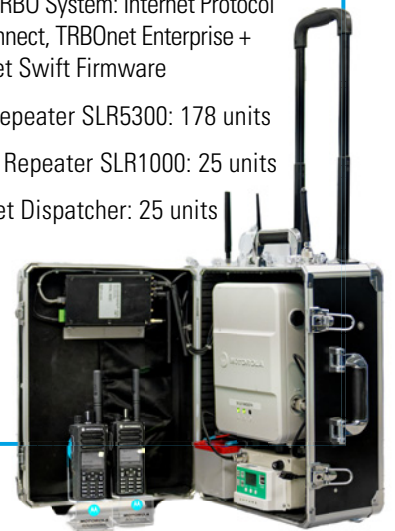
Customized Portable Setup of the Mobile Repeater SLR1000 with a Luggage Case, Battery and 4G Router
