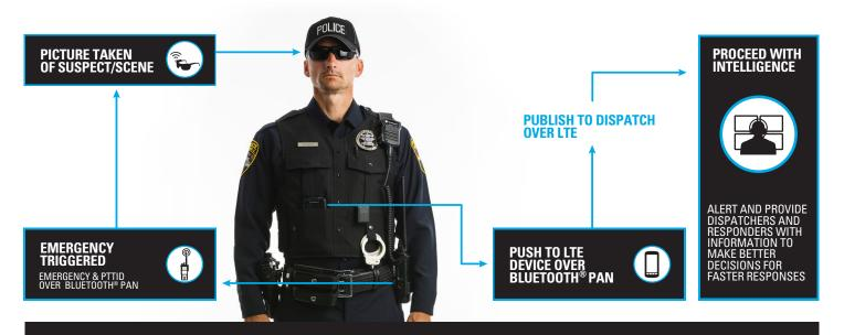
An officer pushes the emergency button on his P25 digital LMR radio, which automatically notifies dispatch and triggers his wearable camera to take a photo of the suspect and the scene. The push-to-talk ID (PTTID) and the photo are sent to dispatch via the officer's Bluetooth® Personal Area Network (PAN) over the LTE network. Dispatch pushes the officer information, location and photo to nearby units who quickly arrive on the scene to provide assistance.
