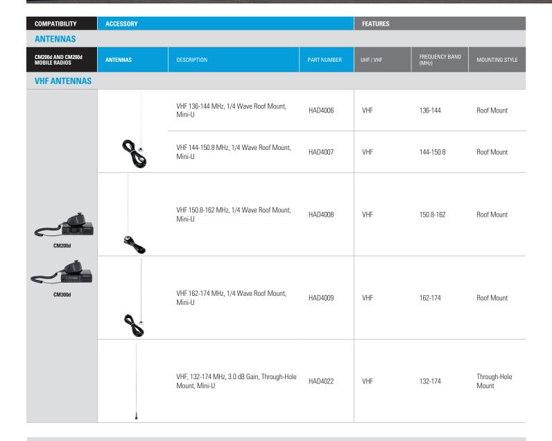
FREQUENCY BAND: Most antennas only cover a portion of a frequency band. Our wideband UHF and VHF antennas offer coverage across the entire band, enhancing your communication flexibility.
