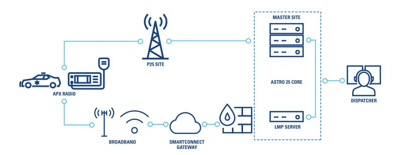
If during the chase the officer returns to P25 coverage, SmartConnect automatically switches the voice channel back to the ASTRO 25 network without intervention by the officer. The switchovers are fast and seamless, with audio remaining on the same talkgroup and radio functionality and voice quality maintained.
