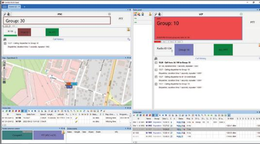
View of the dispatcher console working with two wide-area systems (IP Site Connect and Capacity Plus Multi Site). LOCATION POSITIONING module running. The console shows the use of the function key functionality (direct call to an individual contact or a group).
