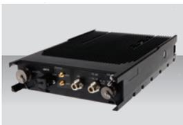
VENDETTA is a highly ruggedized SDR with an integrated PA, receiver circuitry, and a Front End (FE). It is IP-67, rapidly deployable, and can process myriad radio technologies and frequencies.
