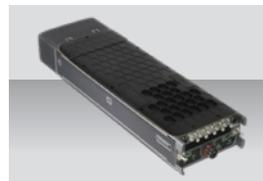
VENOM is a versatile, small-SWaP SDR with a built-in PA, receiver circuitry, and an FE. It is manpackable, compatible with tactical vests and can process myriad radio technologies and frequencies.
