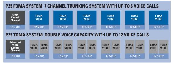
P25 trunking systems with TDMA operation increase their voice capacity with the same number of channels.
