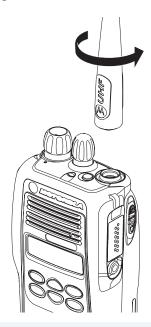
1 Turn the antenna counterclockwise to remove it.
