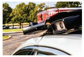
Motorola offers an ALPR Expansion Board for the MW810 that supports up to four Slate<sup>™</sup> digital ALPR cameras from PIPS Technology. Working together, Motorola and PIPS have created an ALPR solution with unparalleled power, intelligence, and flexibility – and without the footprint of a separate ALPR processor.
