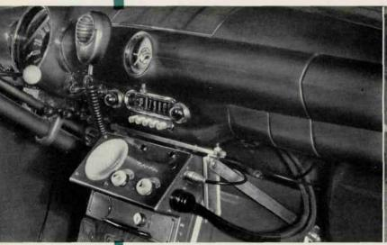
Motorola Uni-Channel Sensicon Dispatcher, one of the newer FM radio mobile communication models, is shown mounted and ready for use in police squad car.
