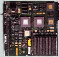
*A single printed circuit board contains the advanced Motorola microprocessors used in the NeXT™ Computer System.*
