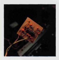
(Above) Key component in Motorola's C-QUAM® AM stereo system is a onechip bipolar integrated circuit that decodes incoming AM stereo signals.
