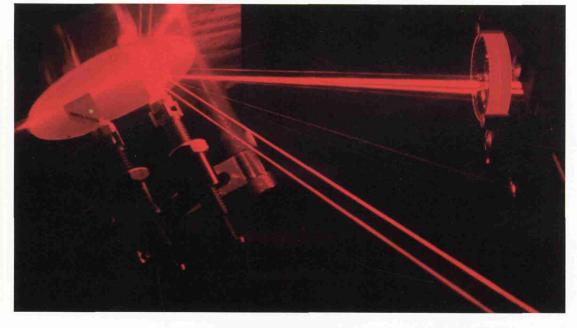
(Above) Meinel optical concentrators proposed for the world's largest solar cell energy plant designed by Motorola for installation at Phoenix International Airport, Ariz., being tested. (Below) A helium-neon laser is being used to develop optical waveguides for eventual use in electronic countermeasures equipment.
