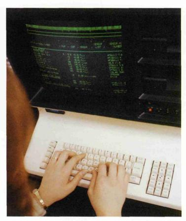
A Motorola 15-inch cathode ray tube (CRT) module is one of the major components of the word processing terminal shown here. The module is a subassembly consisting of a CRT and the electronics required to "light up" data on the face of the tube.
