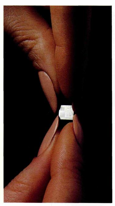
The MC6801 is a single-chip microcomputer that combines the processor, ROM, RAM, clock timer and IO circuits. This chip includes 40,000 transistors.
