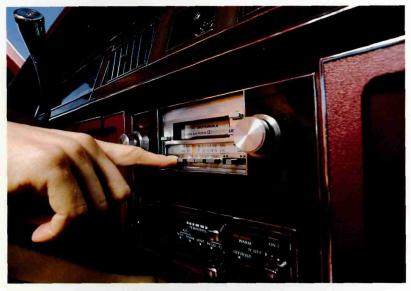
1978 (Above) Motorola's new distributorless ignition system will make an important contribution to both fuel economy and environmental control. (Below) The TC8 90AX, one of the newest autosound systems introduced in 1978. When coupled with our graphic equalizer, it is capable of delivering 30 watts power output and reproducing high fidelity sound in the car.
