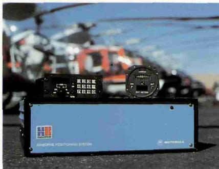
▲ New applications of the Mini-Ranger III™ position determining system include positioning offshore oil platforms and guiding crop and forest air fertilization operations.
