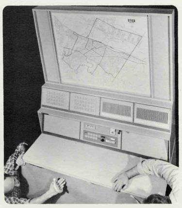
Communications control consoles such as this one being packaged for shipment to the Utica, New York, Police Department must be designed and built for the exact and distinct functional requirements of the users.
