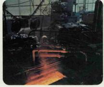
Four housings are made for the electronic alternator through single operation of this 400-ton aluminum die casting machine at the Arcade facility.
