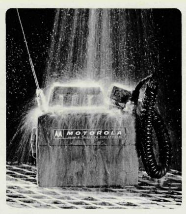
Lightweight 2-way portable radiophones, frequently used in inclement weather by such agencies as police departments, go through dust, cold and rain tests. Rigid standards of reliability are applied to all units.
