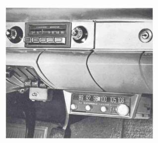
Designed for under-the-dash installation, the new Motorola FM car radio operates independently of or in addition to the car's AM set. The FM-900 can reproduce the entire hi-fi audio range.
