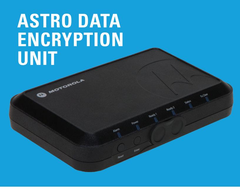
The Data Encryption Unit provides encryption/decryption of P25 data within ASTRO® radio systems. This tamper resistant encryption unit, with integrated physical security, is certified to the National Institute of Standards and Technology FIPS 140-2 Level 3 certification, a very stringent standard for cryptographic modules. The data encryption keys can be centrally managed using a Motorola Key Management Facility (KMF) via Over the Ethernet
