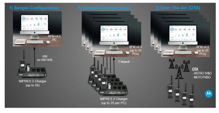
Motorola Solutions' Battery Fleet Management (BFM) V4.0 supports the following three (3) on-prem methods of gathering IMPRESTM battery data:
