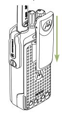
2 To remove the clip, use a flatbladed object to press the belt clip tab (a) away from the radio. Then, slide the clip upward and away from the radio.
