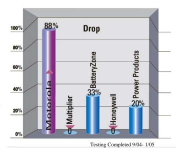
Typical failures included the battery housing splitting, broken latches, being dislodged from the radio or failure to charge.
